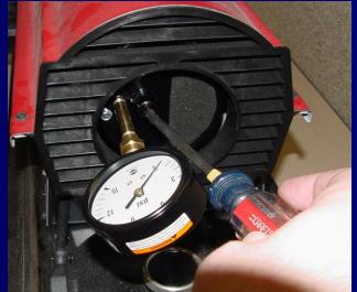
Start the heater and compare the pressure reading to the specified pressure on the data decal. Adjust the pressure relief screw as necessary.
