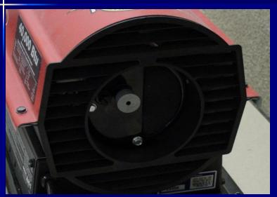
Remove the upper shell and end-cover guard
