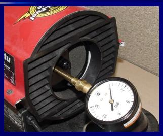
Remove the solid plug on the back of the end cover (left side) and thread in your low pressure 0-15 psi gauge.
