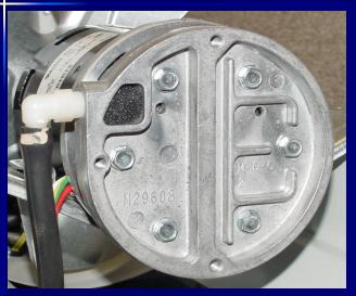
Re-attach the back plate of the pump. Do not over-tighten the screws – over-tightening will damage the threads and can cause a pressure leak.
