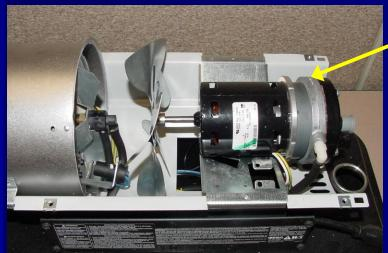
You can now see the pump assembly attached to the back of the fan motor.
