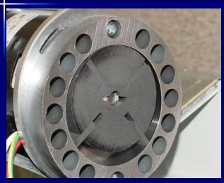
Rotate the rotor slowly with your hand underneath to catch the blades.
